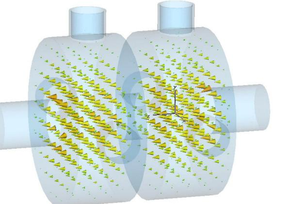
Type = E-Field (peak) Monitor = Mode 1 Maximum-3d = 1.51525e+007 V/m at 0.65625 / 1 / -1.875 Frequency = 1.00027 Phase = 0 degrees
