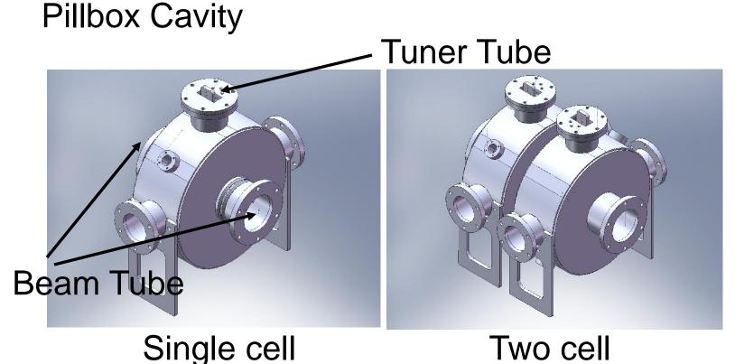
f ~ 1 GHz (TM010), measured Q 1,000 ~10,000 Theory ~19,000. It need a narrow frequency span, no more than a few MHz, to measure a high Q cavity
