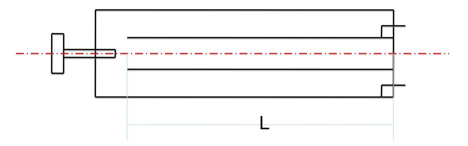
TEM mode, f ~ 350 MHz. Low frequency structure usually for heavy ion (low beta) acceleration
