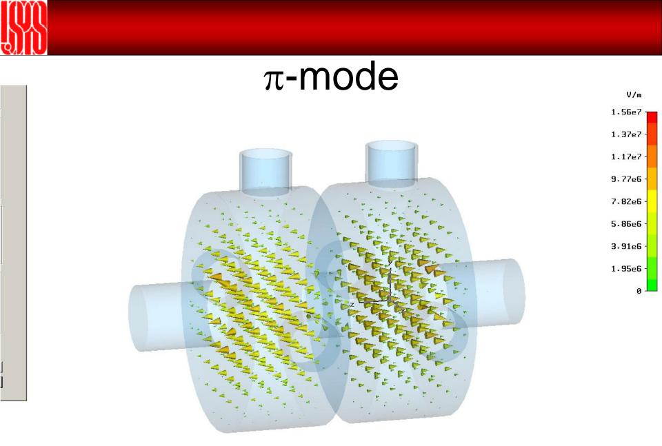
Type = E-Field (peak) Monitor = Mode 2 Maximum-3d = 1.56383e+007 V/m at 0.65625 / 1 / 3.125 Frequency = 1.00169 Phase = 0 degrees
